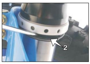
Clean the dust scraper, the outside legs and the rods carefully. Oil them well with silicone spray or with engine oil. Finally, push the dust scraper manually into the outside legs.
