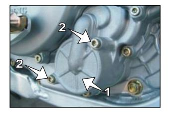
Wait until the oil has drained completely, then clean the sealing surfaces of the transmission cover and filter cover, check the O-Ring and replace it if necessary.
